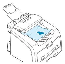
4 Close the control panel. Then load the documents back into the ADF.
